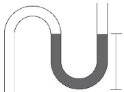
Water trap. Min. 60 mm of standing water
